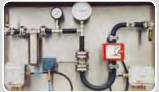
Gas Density Metering Panel Oil & Gas Industry
