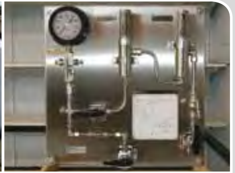
Valve Seat Leak Indicator Panel Oil & Gas
