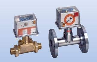
Measuring ranges: Water: 3 - 55 l/min...50 - 600 l/min Connection: Rp  $1\!\!\!/_2\ldots$ Rp 2 female, R $1\!\!\!/_2\ldots$ R 2 male,  $1\!\!\!/_2"\ldots$ 2" NPT Flange: DN 15...DN 50, ASME  $1\!\!\!/_2"\ldots$ 2"  $p_{max}$  16 bar;  $t_{max}$  100 °C Universal mounting Accuracy:  $\pm$ 3... $\pm$ 5% of full scale Flap Flowmeter for Liquids Material: steel, stainless steel, PP, PTFE, Hastelloy
