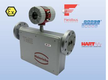
Measuring range: Water: 0 - 60 kg/h ... 0 - 60 000 kg/h  $t_{max}$  180 °C;  $p_{max}$  40 bar/300 lbs Connection: flange DN 10 - 80 /ANSI ½"-3" Accuracy Liquids: ±0.15% of reading ±ZP-stability Gases: ±0.5% of reading ±ZP-stability
