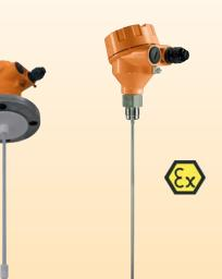
Version: rod, rope, koaxial version Application: liquids and bulk solids  $t_{max}$  250°C;  $p_{max}$  40 bar Connection: thread, flange Analogue output, switching output Accuracy:  $\pm$  3 mm or 0.03 % of measured value Ultrasonic Measurement Material: PP, PVDF Model: NUS-4
