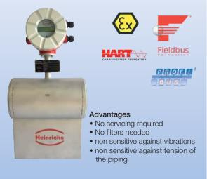
Viscosity range: 0.3 - 50 000 mPas Measuring range: 0 - 120 kg/h...0 - 120000 kg/h Water  $t_{max}$  +260 °C;  $p_{max}$  40 bar/600 lbs Connection: flange DN20 - 100 /ANSI ¾" - 4" Accuracy:  $\pm$  0.1 (0.15) % of reading  $\pm$ ZP-stability
