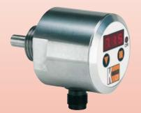
Measuring range: -20...+120°C p<sub>max</sub> 80 bar Connection: G ½, G ¾, ½" NPT, ¾" NPT AG Analogue output, limit contact Accuracy: ±0.5°C
