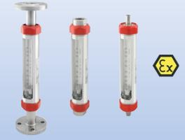
$\begin{array}{l} \mbox{Measuring ranges: Water: $2.5-25...1000-10000 l/h$ \\ \mbox{Air: } 0.8-8...28-280 \mbox{Nm}^3/h$ \\ \mbox{t}_{max} -10...+100 \mbox{°C; } p_{max} \mbox{15 bar} \\ \mbox{Connection: G $14 ...2 female, flange DN $10...65$, \\ \mbox{ANSI $12" ...2 $12", hose connection, glue connection, \\ \mbox{Options: limit contacts} \\ \mbox{Accuracy: Cl. $1.6 / $2.5 according VDI \\ \mbox{Liquids: $1.6 $\%$} \\ \mbox{Gases: $2.5 $\% \mbox{VDE/VDI} \\ \end{array}$
