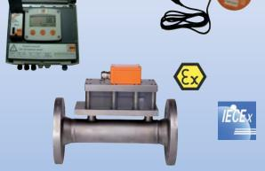
Measuring rage: Air: 0,2 - 20 Nm<sup>3</sup>/h ... 60 - 6000 m<sup>3</sup>/h Pressure Drop: max. 50 mbar t<sub>max</sub> 120 °C (for EX 60 °C); p<sub>max</sub> PN 40 Connection: flange DN 25 ... 200, ANSI 1"... 8" Accuracy:  $\pm 1.5$ % of reading
