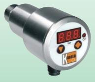
Measuring range: -1 ... 0 bar ... 0 ... +400 bar Display: 3-digit LED Connection: G  $\frac{1}{4}$ , G  $\frac{1}{2}$ ,  $\frac{1}{4}$ " NPT,  $\frac{1}{2}$ " NPT male Accuracy:  $\pm 0.5 - 1$ % of full scale
