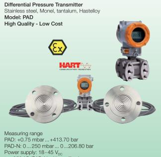
$\begin{array}{l} t_{max} 250 \ ^{\circ}C \ (PAD-N \ with \ capillary) \\ \hline Connection \\ PAD: 14" \ NPT, 1/2" \ NPT \\ PAD-N: flange-, thread-, clamp on-, and in-line diaphragm seal \\ (nominal size 15...100) \\ Accuracy \\ PAD: \pm 0.075\% \ of \ measuring \ span \\ PAD-N: \pm 0.075\% \ of \ calibrated \ span \ + \ influence \ of \ diaphragm \ seal \\ \end{array}$
