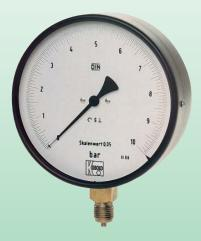
Measuring range: -0.6...0 bar...0...+2500 bar Housing: Ø 160, 250 mm Overload protected:: 1,0 times - (calm) Connection: G  $\frac{1}{2}$  male Accuracy: Cl. 0.25; 0.6
