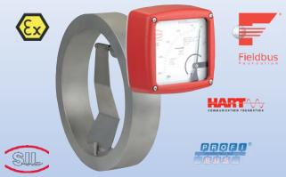
Measuring range: Water: 0,5 - 3,5 m³/h...200 - 1500 m³/h t<sub>max</sub> -40...+300 °C; p<sub>max</sub> 40 bar, from DN 100: 16 bar, from DN 200: 10 bar, higher on request Connection: wafer flange DN 25...500, ANSI 1½"...20" Options: limit contacts, analogue output, HART®, Profibus® PA, Fieldbus® Foundation™ Accuracy:  $\pm 2.5\%$  of full scale
