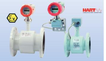
Measuring range: Water: 0 - 10 m/s 1 ... 40300 m<sup>3</sup>/h Min. conductivity Liquids in general:  $\geq 5 \,\mu$ S/cm Demineralised water:  $\geq 20 \,\mu$ S/cm t<sub>max</sub> 150 °C p<sub>max</sub> 40 bar Connection: flange DN 10 - 1 200/ANSI ½" ... 48" Outputs: analogue output, HART<sup>®</sup>, pulse and status Accuracy:  $\pm 0.3 \%$  of reading  $\pm 0.01 \% \times Q_{max}$
