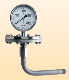
Measuring range: 0 - 600 ... 0 - 10 000 mmWS  $t_{max}$  80 °C Connection: G  $1\!\!\!/_2$  male,  $1\!\!\!/_2$  " NPT, DN 50 ... 100, ANSI 2" ... 4" Accuracy:  $\pm$  1.6 % of full scale
