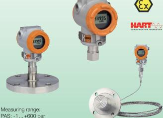
PAS: -1... +600 bar PAS-N: 0... +350 mbar ... 0... +600 bar t<sub>max</sub> 200°C (PAS-N with capillary) Connection PAS: ½" NPT female PAS-N: thread or with flange (nominal size 15... 100) Temperature: -40... +120°C (diaphragm seal up to 250°C) Accuracy PAS: ±0.075% of calibrated span PAS-N: ±0.075% of calibrated span + influence of diaphragm seal
