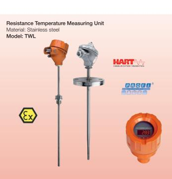
Measuring range: -80... +600 °C  $p_{max}$  250 bar Connection: thread, flange, weld-in sleeve Output: analogue output, resistance, Profibus® PA Option: digital display Pt 100, 4...20 mA Accuracy: Cl. A or B
