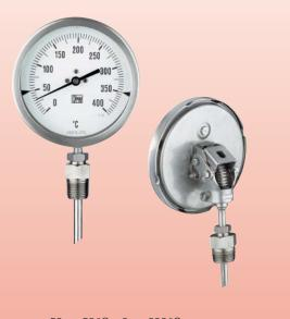
Measuring range:: -50...+50 °C...0...+600 °C  $p_{max}$  15 bar Connection: G  $\frac{1}{2}$ ... $\frac{3}{4}$ ,  $\frac{1}{2}$ "... $\frac{3}{4}$ " NPT, fixed, rotatable, slidable Accuracy: Cl. 1,0
