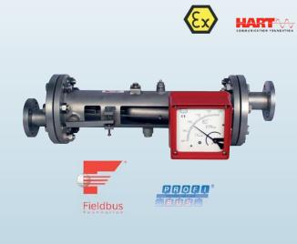
Measuring range: 700... 1 900g/l Measuring span: 50... 600 g/l Flow: max. 2 500/5 000/10 000 l/h t<sub>max</sub>150 °C; p<sub>max</sub> 16 bar/150 lbs Flansch DN 25... 50, ANSI 1"...2" Options: limit contacts, analogue output, HART®, Profibus® PA, Fieldbus® Foundation<sup>TM</sup> Accuracy:  $\pm$  1.25 - 6.0 g/l according to span
