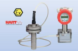
Measuring range: Water: 0 - 10 m/s  $t_{max}$ 100 °C;  $p_{max}$  PN 16 Connection: weld-on nozzle Ø 40 mm, sensor with union nut M52x2 for pipelines DN 50...400, ANSI 2"...16" IP 68 Accuracy:  $\pm$  1.5 % of full scale Magnetic Inductive Flowmeter - INSERTION-version -Material: stainless steel, PFA, PTFE Model: PIT
