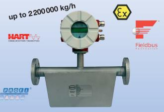
Measuring range: 0 - 60 kg/h...0 - 2 200 000 kg/h  $t_{max}$  +260 °C;  $p_{max}$  40 bar/300 lbs (up to 750 bar on request) Connection: flange DN 10-400 / ANSI, JIS Accuracy Liquids: ±0,1% of reading ±ZP-stability
