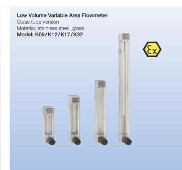
Installation lengths: 90 mm / 125 mm / 175 mm / 320 mm Measuring-/switching ranges: Water: 0.02 - 0.25... 10 - 100 l/h Air: 2 - 20... 300 - 3000 Nl/h t<sub>max</sub>: 0... + 100 °C, (0... + 70 °C with contact); p<sub>max</sub>: 16 bar Connection: G ¼, G ½, ¼ " NPT, Swagelok, Ermeto
