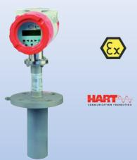
Measuring range: Water: 0,5 - 5 m/s oder 1 - 10 m/s  $t_{max}$  -40...+140 °C;  $p_{max}$  40 bar Connection: flange DN 40...80, ANSI 2"...3", for pipelines DN 125...2000 weld-on connection for pipes DN 125...2000 analogue output, HART®, pulse and status Accuracy:  $\pm$ 1.5 % of reading, +0.5 % of full scale
