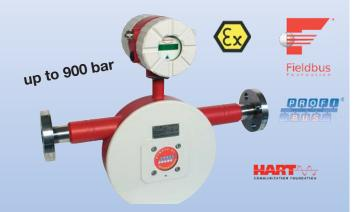
Measuring range: Water: 0 - 0.8 kg/h ... 0 - 65 000 kg/h t<sub>max</sub> +260 °C; p<sub>max</sub> 40 bar (up to 900 bar on request) Connection: flange DN 10 - 100; ANSI ½" - 4"; JIS, NPT Accuracy Liquids:  $\pm 0,1$ % of reading  $\pm$ ZP-stability
