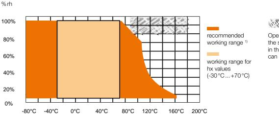
Operating the sensor in these areas can damage it!
